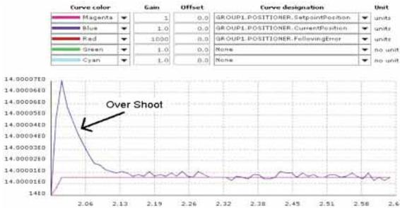
For the image above, the current position has an appreciable overshoot compared to the RMS noise further in the motion profile. Decreasing  $K_p$  will reduce the overshoot.
