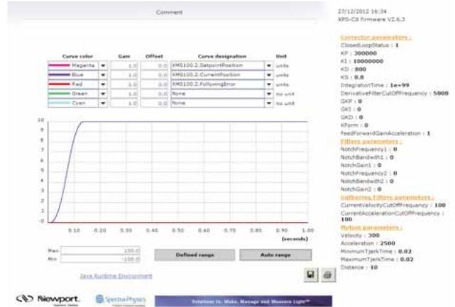
In the chart above the ordinate (Y) axis is in the XPS units of mm whereas we expect the following error to be on the order of microns. Enter of gain of 1000 for the following error in order to have the following error plot display microns on the existing mm scale.
