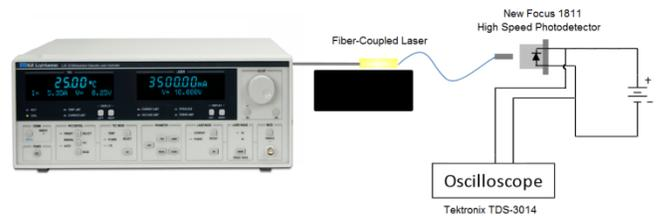
Figure 4: Schematic of transient testing of the LDC-3736 Quantum Cascade Laser Controller
