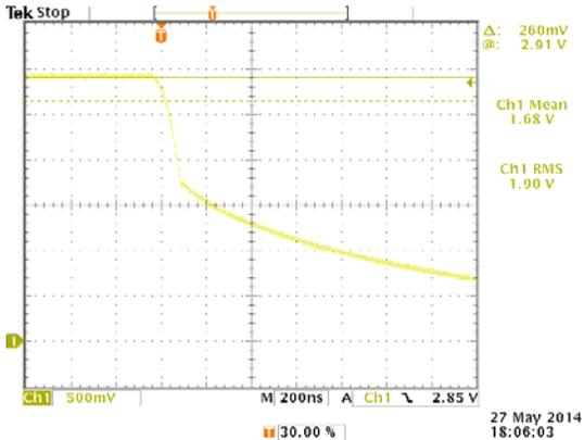
Figure 5: LDC-3736 laser current disabled due to loss of power or brown out
