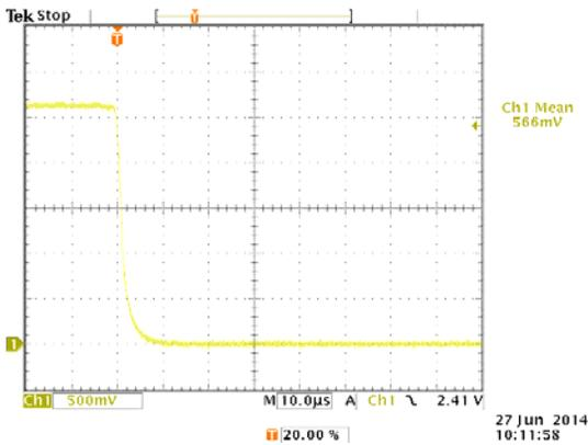
Figure 3: Fast shut down response of the LDC-3736
