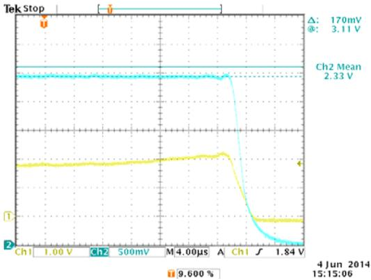
Figure 8: Intermittent contact response of the LDC-3736 with appropriate voltage limit setting
