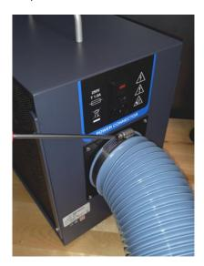
5. Place the filter element flush against the ozone eater opening. There are two filter elements; one is mounted to each opening. These filters may come pre-installed from the factory.
