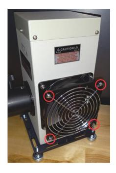
3. Put the lamp housing flange adapter supplied with the 66087 in place of the fan guard and replace and tighten the four screws and nuts<sup>1</sup>, as shown in the photo below.
