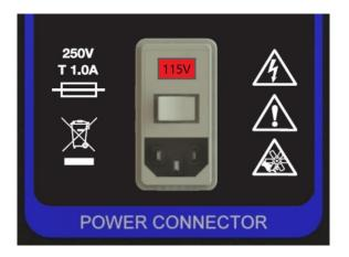
The 115/230 switch above the socket should be set to the 115V position before plugging the line cord into the 115V power source, as shown in the above graphic with the 115V indicator visible through the window.
