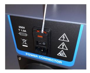
After opening the cover, the voltage selector / fuse box can be removed in a similar fashion, gently prying first with the tool in the recessed slot, before pulling straight outwards from the unit when it is accessible.
