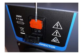
The two 5 x 20 mm fuses should be placed on the innermost terminals, on either side of the fuse box, as shown in the images below.
