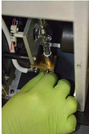
Figure 12: Tightening thumbscrew
