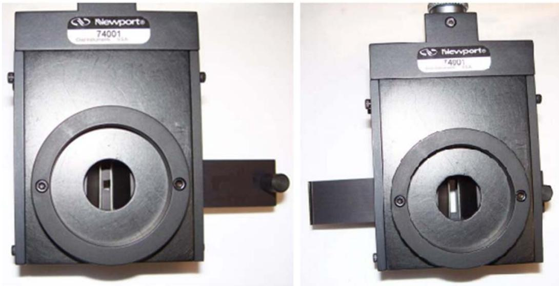
**Figure 76: Using the slide to adjust the micrometer driven slit to its minimum (left) or maximum (right) height**
