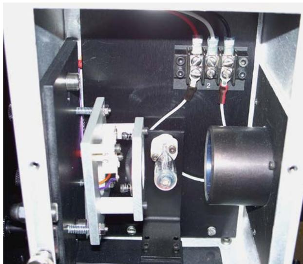
**Figure 14: QTH lamp installation**
