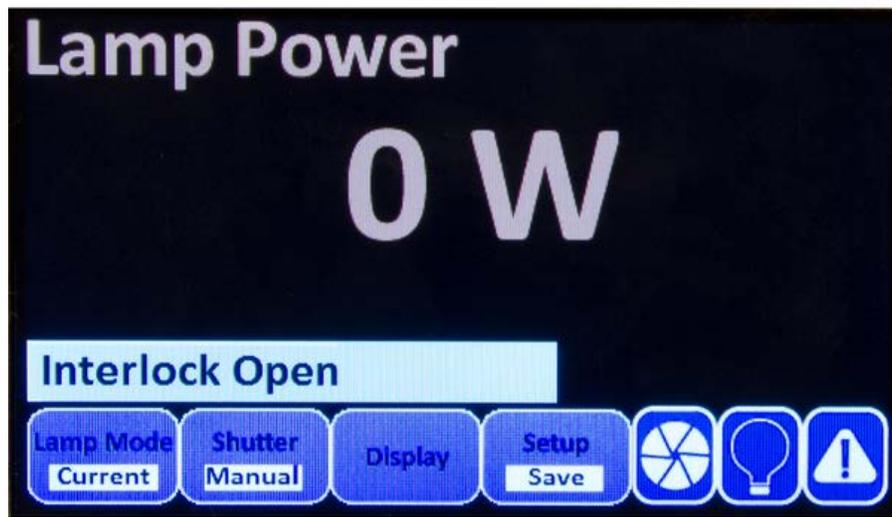
Figure 11: Interlock Open Error Message of the OPS Series Power Supply
