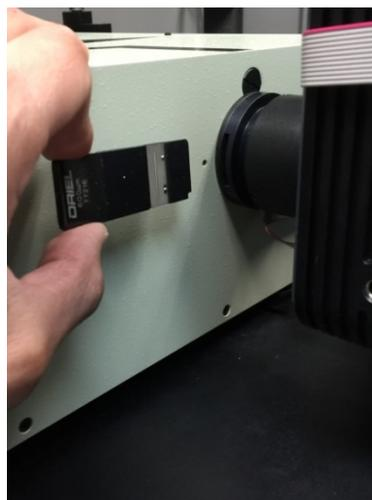
**Figure 73: A 600  $\mu\text{m}$  fixed slit oriented properly for installation**
