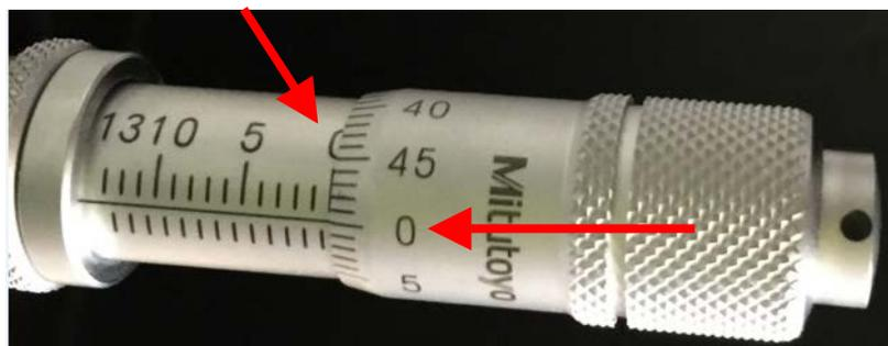
**Figure 75: A micrometer at fully closed slit setting**
