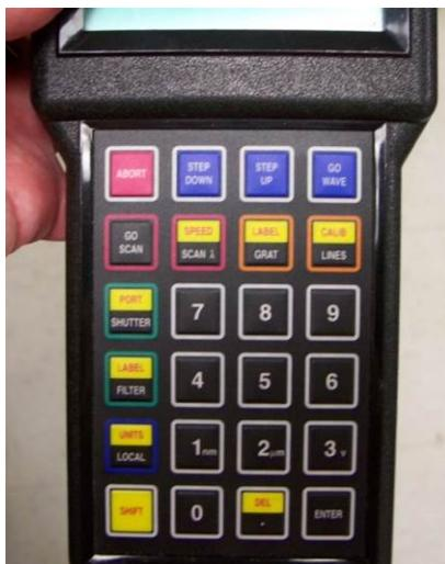
Figure 97: 74009 Monochromator Hand Controller
