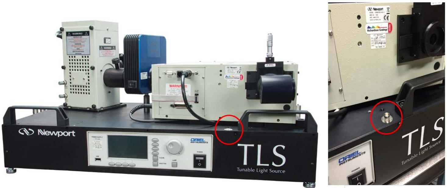
**Figure 83: The BNC connector on the TLS260 baseplate for detector readout**
