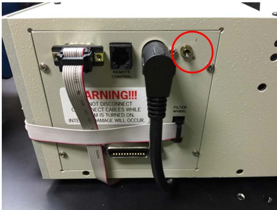
Figure 3: The On/Off switch of the Cornerstone 260 monochromator
