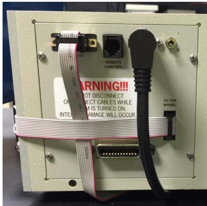
**Figure 88: AC Power and component connections to the Cornerstone 260 monochromator**
