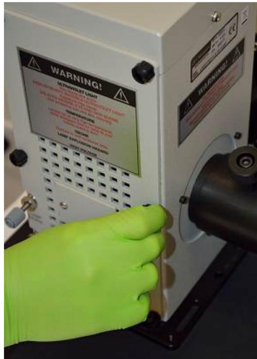
**Figure 5: Opening lamp housing door**
