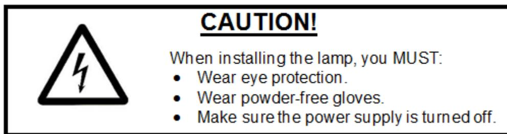
Read all warning labels and literature that were provided with the lamp and all literature provided with this system. The power supply must be unpowered before installing the lamp. Never touch the envelope of any lamp. If it is touched, clean it with isopropyl alcohol and a lint-free tissue such as a Kimwipe®.
