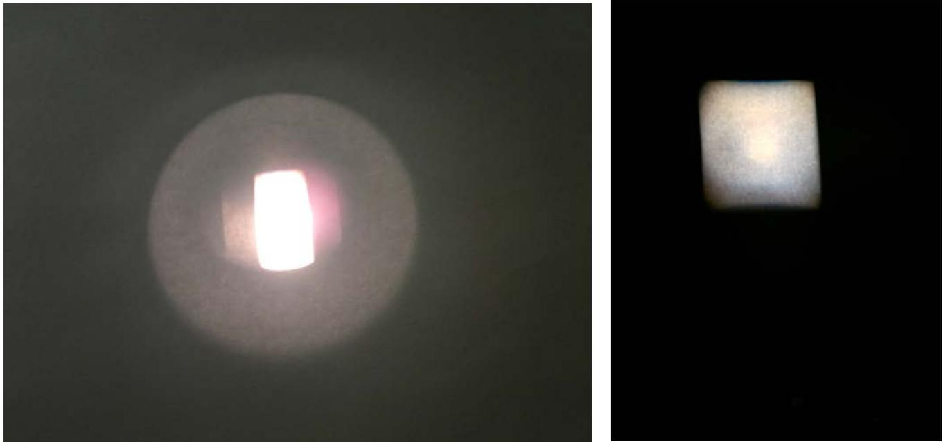
Figure 71: Uniform output of a properly aligned Xe lamp
