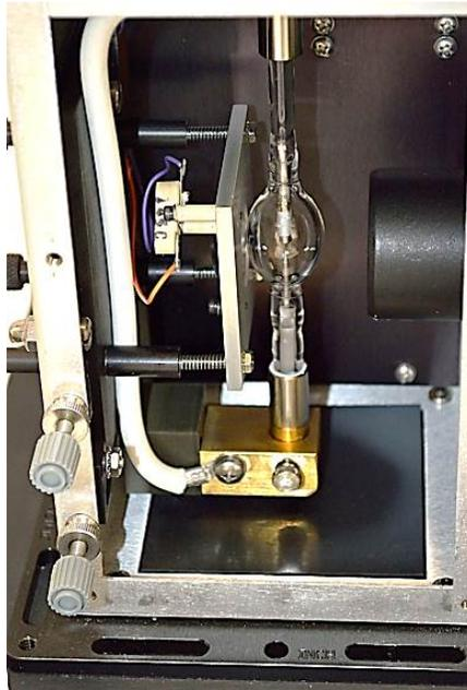
**Figure 13: Xenon arc lamp installed**
