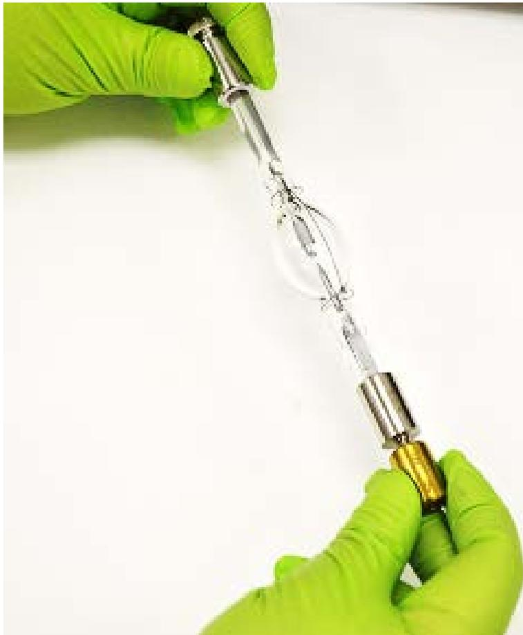
**Figure 7: Socket adapter installation**
