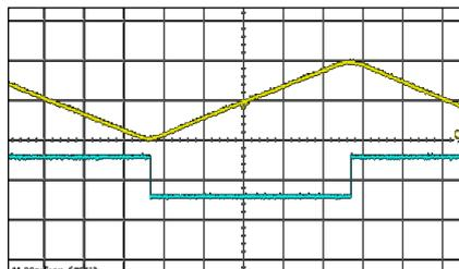
Function  $trgedge,7$ : at any change of moving direction a trigger with length  $n * 20\mu\text{s}$  appears (parameter  $n$ :  $trglen$ ).
