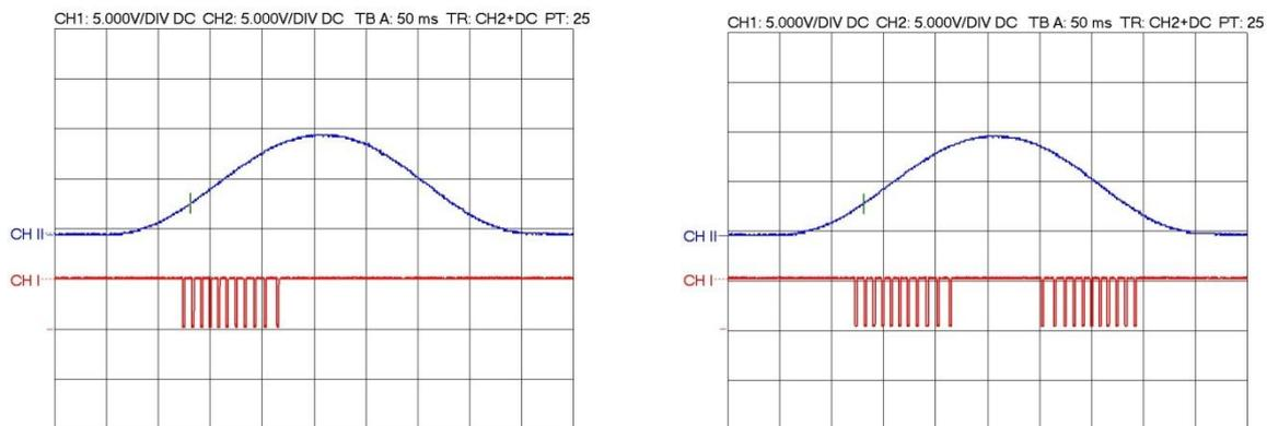
*sketch 6: sine scan with trigger impulses at rising / both edges*
