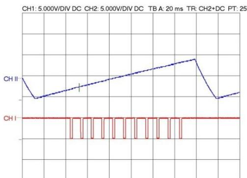
*sketch 7: triangle scan with trigger impulses at the rising edge*
