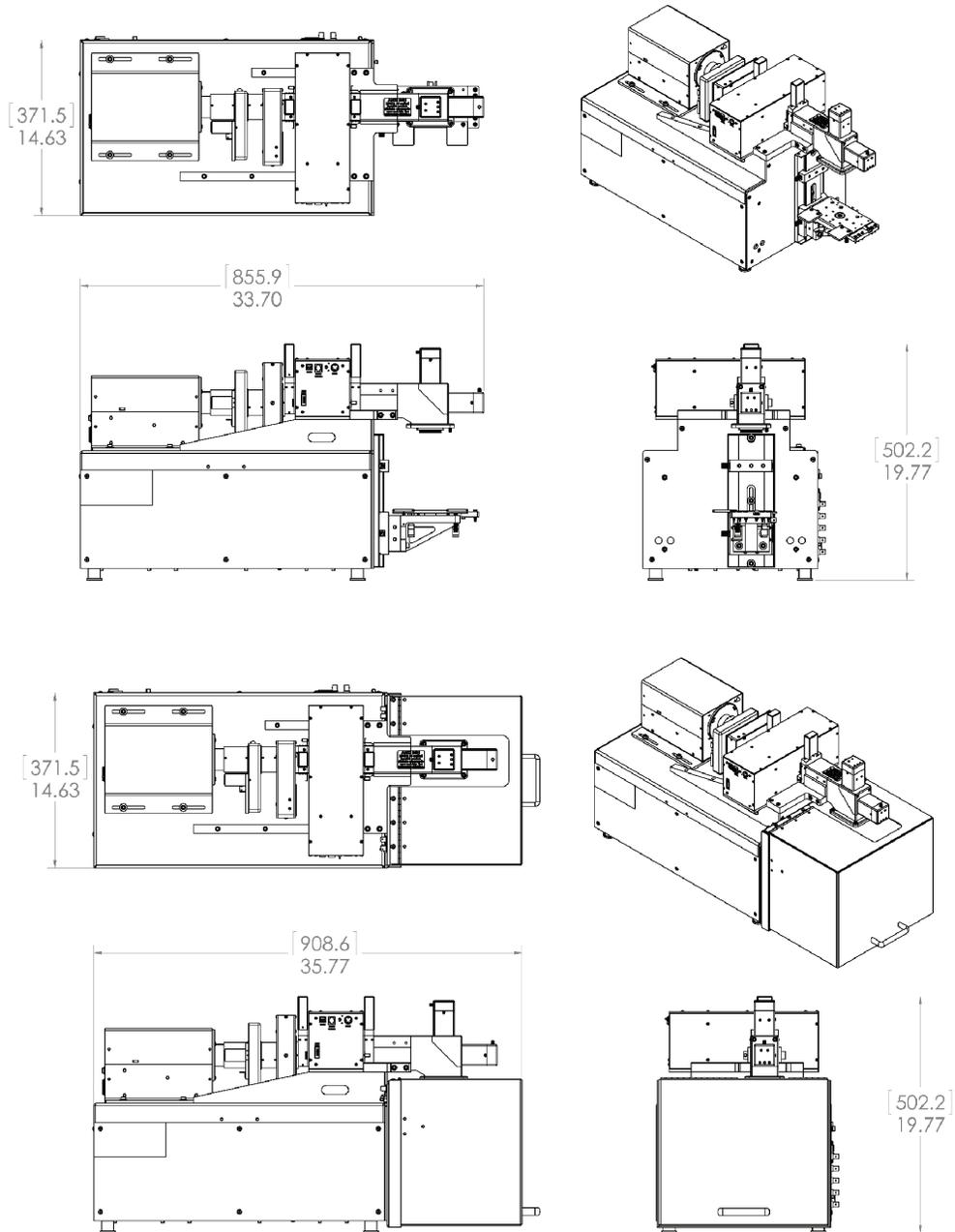
Note that the actual monochromator used in this product is not accurately reflected in the diagrams above, but the overall system dimensions remain unchanged.
