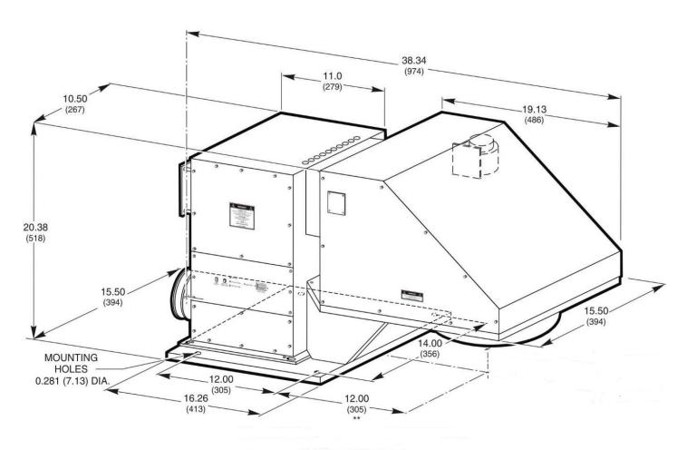
\*\* THE DISTANCE FROM THE CENTER OF THE BEAM PATH TO THE CENTER OF THE MOUNTING HOLE.
