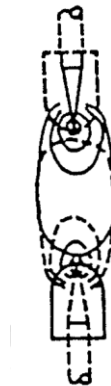
Figure 19 : Correctly positioned reflector overlays the inverted arc image on the arc gap. The image is the same size as the arc itself.
