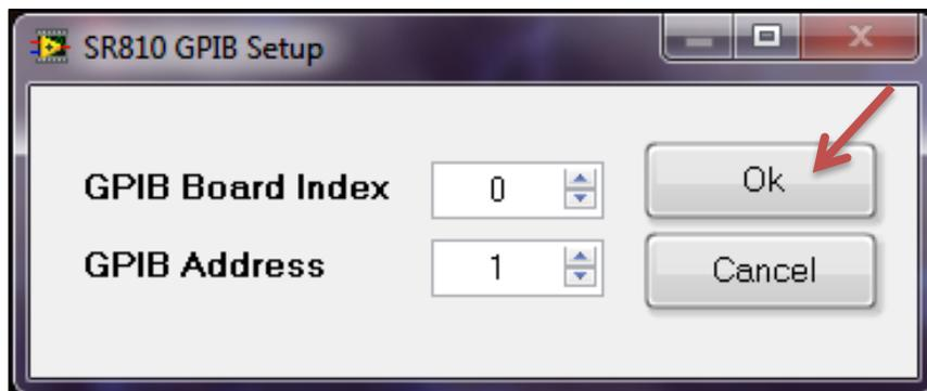
Figure 125: LIDA GPIB Communication Setup.
