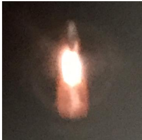
Figure 45: Xe arc lamp output with primary arc image centered.
