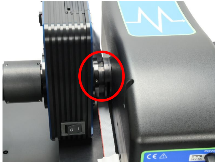
Figure 31: The fixed slit holder at the input port of the monochromator.
