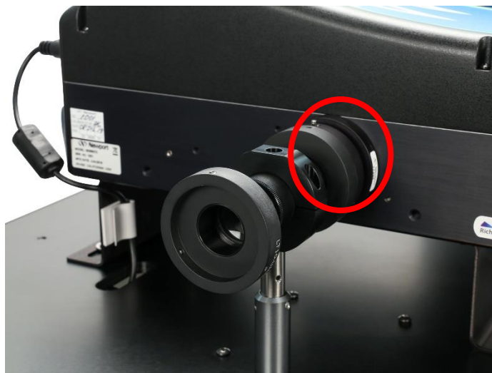
Figure 32: The fixed slit holder at the output port of the monochromator.
