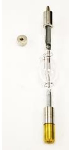
Figure 9: Lamp Prepared for Installation
