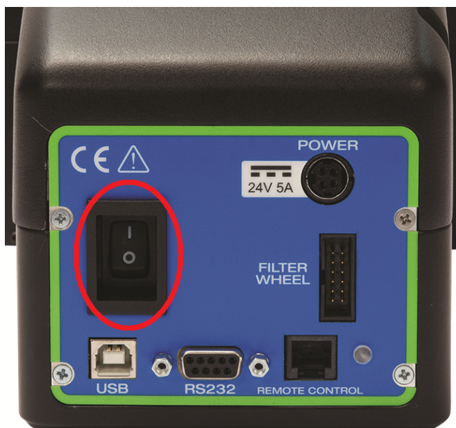
Figure 4: The On/Off switch of the Cornerstone 130B Monochromator circled in red
