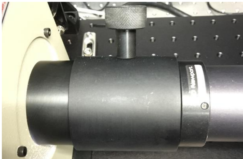
Figure 37: Condenser lens assembly adjustment knob and adjustment lever at output of lamp housing.
