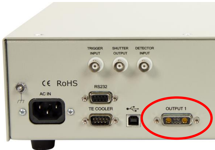
Figure 18: Power Supply Connections
