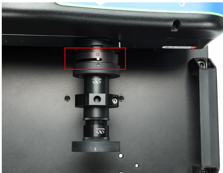
Figure 48: Manual iris added to the output optics of the TLS.
