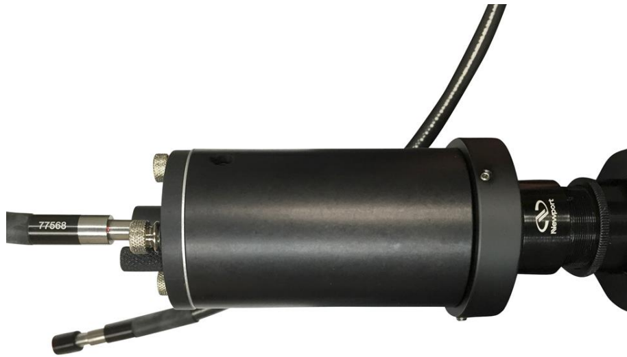
Figure 51: Fiber bundle coupled to the output of the TLS with a fiber bundle focusing assembly.
