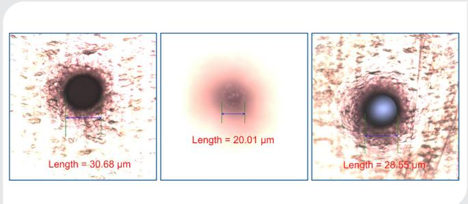
Figure 1. Blind via in Cu/MPI/Cu laminate with microscope focus on the top copper (left) and bottom copper (middle); through-hole via imaged at the top copper surface (right).
